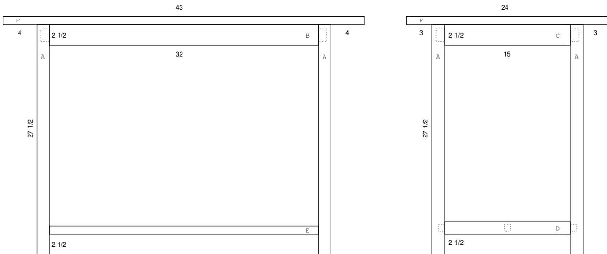
The base construction is mortise and tenon joinery and the table top can be held to the base using any method that allows for wood movement. I will probably use buttons that ride in a groove in the top rails.
